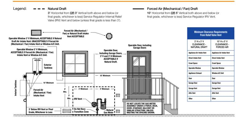
The preferred meter assembly location shall be at the front corner, along the front wall of the structure, or within 3 to 5 feet along either side wall from the front of the structure. On the garage side, the meter location shall be on the front side wall.
