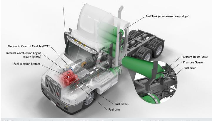
This illustration shows a typical heavy-duty, Class 8 CNG truck. The various components of the CNG fuel system are highlighted. *Illustration by Josh Bauer, NREL*
